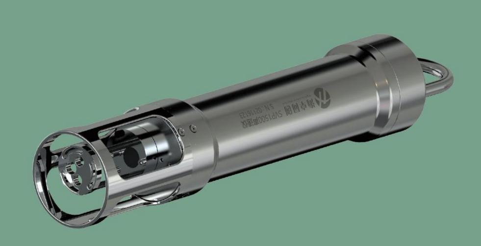
Sound velocity profiler is widely used in many applications including marine survey, underwater construction, underwater terrain mapping, underwater navigation and positioning. SVP1500 sound velocity profiler adopts "time leap" technology for sound velocity measurement. The sound velocity measuring accuracy reaches 0.05m/s. It has integrated a high-precision pressure sensor. The depth accuracy can reach 0.15m, which had reached the world leading level.
