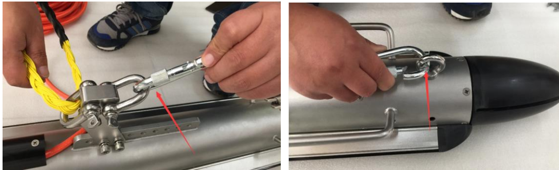
Figure 5.10 Safety Cable Installation
