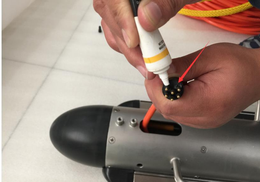
Figure 5.5 Apply Waterproof Silicone Grease
