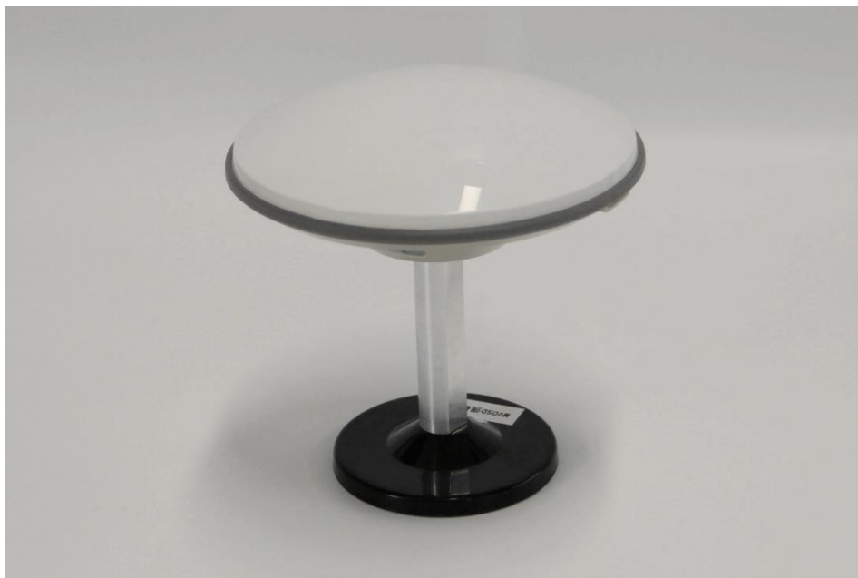
Figure 6.5 GNSS Antenna and Magnetic Mounting Pole
